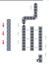
Independent of the process, the empty tubes on peg trays are returned on a conveyor belt in longitudinal direction at the rear of the machine.
