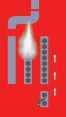
**1 | GENERATION OF VACUUM** The steam area is steamed and emptied several times to reach the required vacuum / remaining oxygen content.
