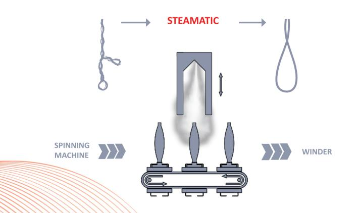
The Steamatic automatically takes over the cops (bobbins) on the peg trays directly from the exit of the spinning machine and transports them under the steam dome. After steaming, the cops are conveyed smoothly to the winding machine. This is done simultaneously, with one peg tray carrier being loaded, one being processed and one being emptied at the same time.
